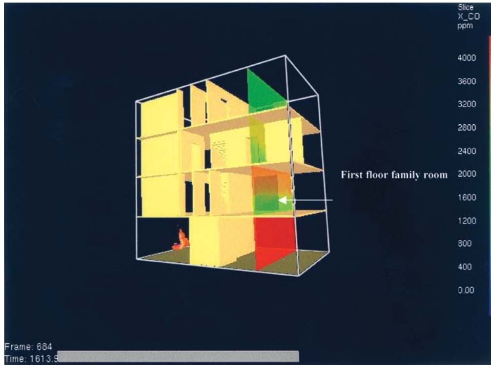
FIG. 1—Modeled fire 27 min after ignition.
